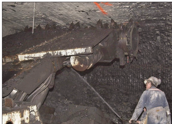
An Eimco 2810-3 continuous miner in operation at the Buckingham Coal Co., Inc., underground coal mine in Athens County, Ohio.
